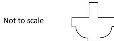
As described below, a new muntin profile was introduced when the tavern was built, reportedly in 1804. With the exception of the single attic sash shown above, all sashes in the Cape Cod house were changed to the new profile at that time. New fenestration includes the sidelights of the front door of the older house.
